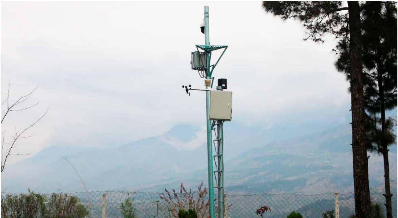
Fire detection camera and automatic weather station towers at the pilot installation site, Kaghan Forest Division, Mansehra
